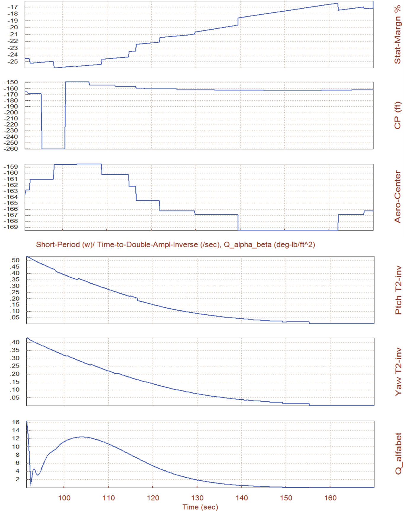
Static Margin, Center of Pressure, Aero-Center (ft), Zulu Launch Vehicle, Second
